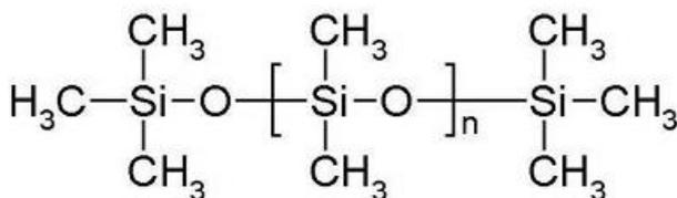
WACKER® AK 350 is a linear, non-reactive polydimethylsiloxane with a viscosity of approx. 350 mm<sup>2</sup>/s. Due to its chemical structure, WACKER® AK 350 has an outstanding property profile, which sets it apart from organic materials such as mineral oils.
